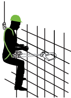
FIGURE 7 - PROPER USAGE WHEN POSITIONING ON VERTICAL REBAR
